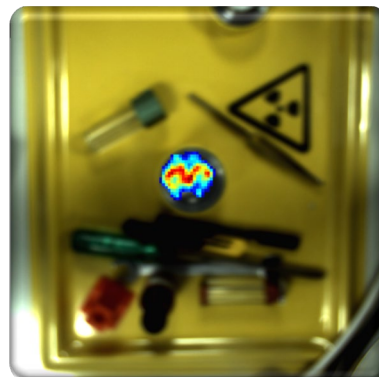
Precise localisation of a 5mm diameter americium-241 source (12.5 MBq, 60 keV) in a lead pot (lid removed)
